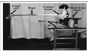
**Figure 3:** Experimental setup for measurement of back muscle strength.
